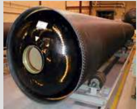
GEM cases are produced using advanced filament winding techniques developed and refined by Northrop Grumman for over 40 years
