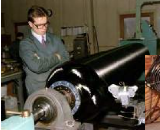
Graphite-Epoxy Composite Case Winding (21-in. booster)
