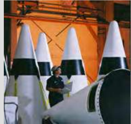
Northrop Grumman uses proven hand layup techniques to produce GEM 60 nose cones
