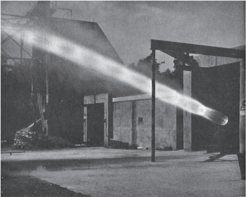
FIGURE 2 This is what a test firing should look like. Note the mach diamonds in the exhaust stream. U.S. Navy photo
